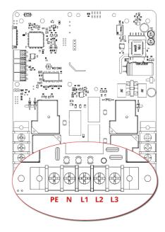
**5)** After completing the electrical connection, the housing can be placed on the back plate. If the white ribbon cable has been disconnected, reconnect it. The cable is placed in the connector with the contacts facing up.
