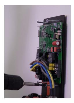
Thread the power cord through the left gland. Do not tighten the gland yet. Place hose clamp (supplied with the device) on the cord and tighten it just enough to eliminate movement.
