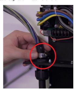
3. Remove isolation from the power cord. Remove enough of it to free around 15 cm of smaller cords. Remove isolation from them as well and using proper tools finish them with fork terminals (supplied with the device). Remember to adjust the length of the cords so that there will be only required minimum of them inside the device. Leaving the cords too long will cause problems with closing the device as the cords wil interfere with casing.
