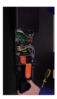
It is advised to remove the white ribbon from the socket on charging controller before mounting the charger on the wall. It will allow to remove the casing completely. Thanks to this it can be protected from being damaged during installation.
