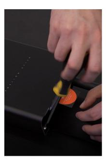
2. Carefully start removing the casing. Proceed with extra caution after revealing white ribbon.
