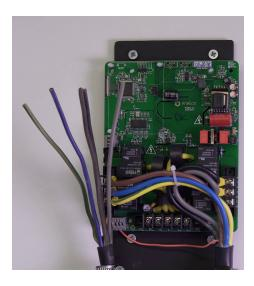
4. Start screwing the fork terminals into right poles in the terminal barrier block. This operation must be performed with extreme caution. Always make sure the cords are being placed in right poles.
