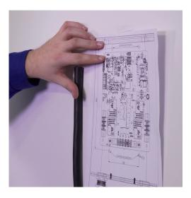
The cord will be completed with the fork terminals supplied with the device during the installation process. Having that in mind please leave the cord unfinished (open ended) for the time of installation.
