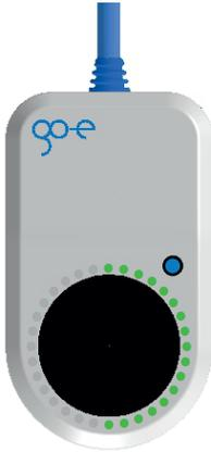
After an initial self-test, the LEDs light up in the number of the pre-set charging current in amps. The setting knob (5) can be used to select between 6A and 32A. The levels of the selection can be individually adjusted in the app. It does not matter whether the go-eCharger is connected in one or three phases.
