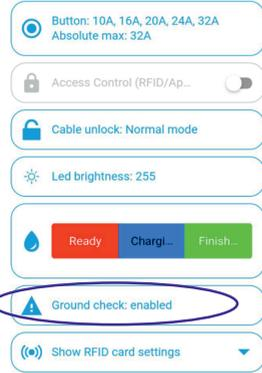
Attention: This function should only be used if the mains supply has no grounding (IT mains). If you are not sure, leave the setting to "Ground check enable"!
