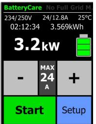
No Full Charging can be switched on via Setup menu, while BatteryCare is enabled. This function is preventing your battery to be fully charged. Once finalising (constant voltage) phase is detected, car charge stops. For your information status "No Full" stays orange until reset with Start button.
